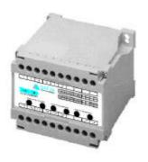
The T25-LF frequency transducer converts AC voltage to a linear DC output signal proportional to the frequency of the input. Employing a crystal based oscillator conversion principle, the measured frequency band is accurately represented by proportional linear DC voltage or current output.
